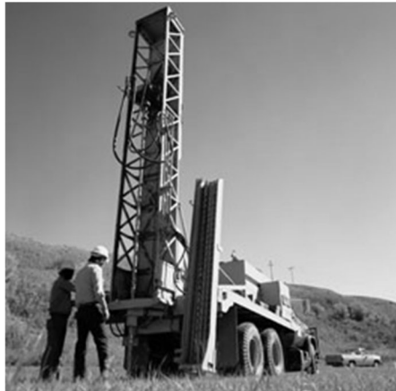
Operators preparing a hole for the explosive charges used in seismic exploration Source: Stock photography (copyrighted)
